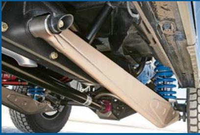
In addition to the cool-running shocks and fade-free shock ratio, the complete rear suspension is mounted to a single crossmember that Tom dubbed "The Gauntlet." The Gauntlet is designed to take all of the force generated by the rear suspension, transferring none of it to the frame.
