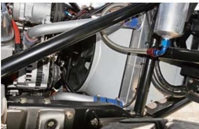
▲ Big ponies put out big heat, so a Ron Davis aluminum radiator sits up front to supply the chill. Tom's TIG-welding expertise also includes aluminum: He built the radiator shroud and sectioned the aluminum radiator tubing.
