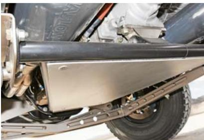
▲ As previously stated, this truck was designed to be easy to work on. If the Ken Mogi-built C6 needs to be dropped for maintenance, the entire framework and skidplate beneath it can easily be unbolted for access. A pair of MagnaFlow mufflers quiets down things while preserving the throaty note produced by the 650 ponies under the hood. The mufflers bolt to custom SI headers.
