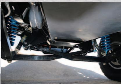
▲ Tom tied the tranny crossmember into the radius-arm pivot brackets, then connected it to the suspension/engine crossmember. This structural bracing is hidden by a custom aluminum skidplate, which keeps the 400 small-block and the TH400 from getting smacked by errant rocks.
