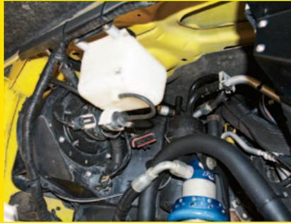
▲▶ Extra tire clearance was built into the front end by cutting and patching the air conditioning case as well as the air filter housing. The execution is so clean it looks factory.
