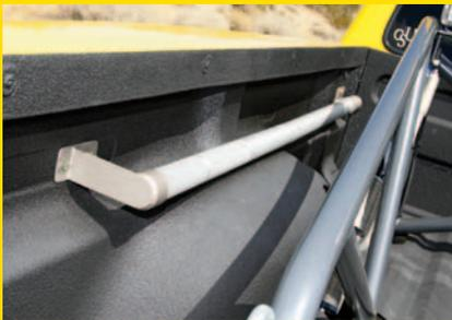
▲ No floating floor jack handles on this truck! Custom brackets keep things secure and easily accessible when needed.
