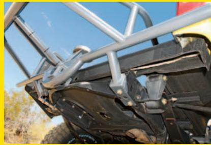
▲ The rear bedcase-and-bumper combo is a joint effort by Dixon Bros. Racing and S.I. Motorsports. The main structure is by Dixon, and S. I. added custom touches in the form of the hitch receiver and the tire carrier.
