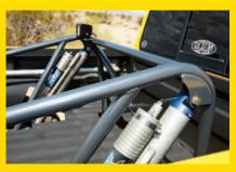
▲ A pair of Fox bypass shocks controls 16 inches of rear wheel travel.
