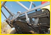
▲ The rear bedcage-and-bumper combo is a joint effort by Dixon Bros. Racing and S.I. Motorsports. The main structure is by Dixon, and S. I. added custom touches in the form of the hitch receiver and the tire carrier.
