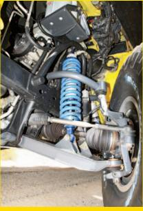
▲ A Dixon Bros. long-travel kit leads the way. This kit ties into stock A-arm pivot points and provides 14 inches of fully functional 4x4 wheel travel. Fox 2.5-inch coilovers with an 8-inch stroke and fourinch-stroke Fox bump stops provide the springing and damping control. Dixon Bros. shock hoops complete the picture.
