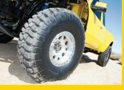
◀ Here's a wheel and tire combo we've seen before: KMC Enduro Beadlocks wrapped with BFGoodrich KM2 Mud-Terrain tires. This is a strong combination that affords traction over a variety of surfaces: perfect for a triple-duty truck.
