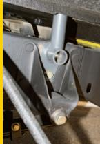
the frame and the bolted brackets. This in turn makes the chassis live a longer, crack-free life.
