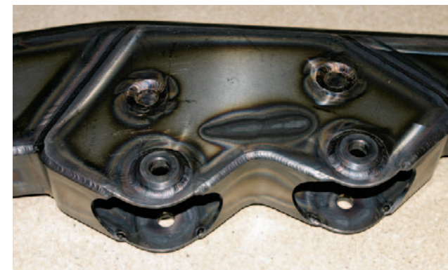
▲ A close look at the shock mounts on the lower link reveals flawless TIG-welding and a simple, effective design.
