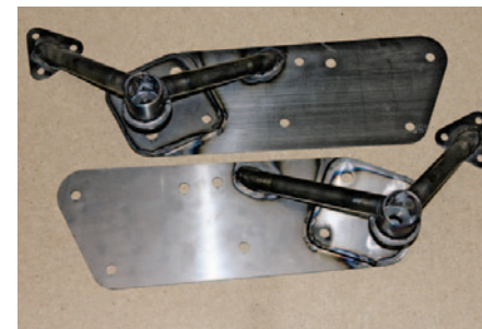
▲ The Plank four-link kit from S.I. Motorsports includes upper and lower links, all hardware shown, bolt-on link-mounting brackets, Delrin pivot bushings for the forward end of the lower links, and weld-on tabs for the rear axle. This system is designed to be used with a Ford 9-inch rear axle. S.I. can truss and tab your axlehousing as an extra-cost option. The links and mounting brackets are all made from 4130 chrome-moly tubing and plate. The system's geometry has been optimized for correct instant center and antisquat and cycles through 28 inches of clean suspension travel. A sway bar is not mandatory with the Plank four-link. The kit bolts to '86-'97 2WD and 4WD SuperCab Ford Ranger pickups using factory frame holes as mounting points.
