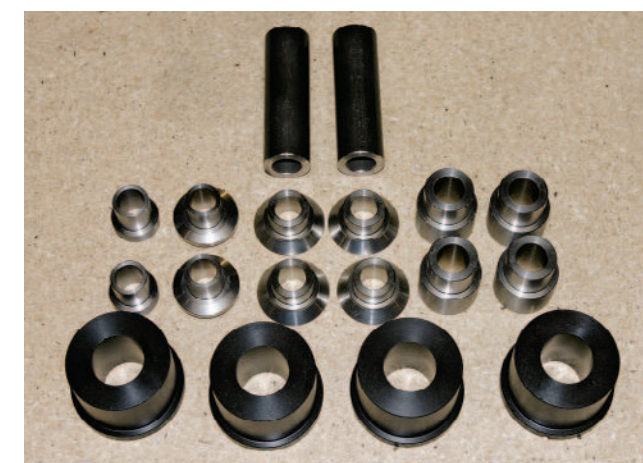
▲ Custom-machined hardware indexes into industry-standard rod ends. The frame-end lower link pivots are crafted from Delrin and are also included.
