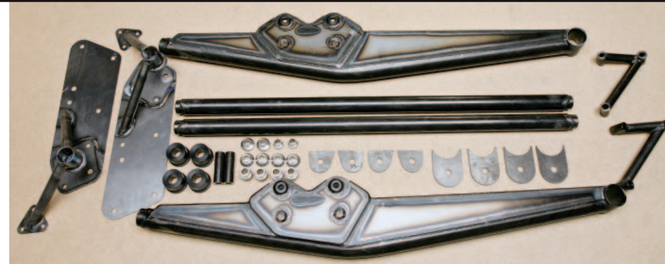
▲ The Plank four-link kit from S.I. Motorsports includes upper and lower links, all hardware shown, bolt-on link-mounting brackets, Delrin pivot bushings for the forward end of the lower links, and weld-on tabs for the rear axle. This system is designed to be used with a Ford 9-inch rear axle. S.I. can truss and tab your axlehousing as an extra-cost option. The links and mounting brackets are all made from 4130 chrome-moly tubing and plate. The system's geometry has been optimized for correct instant center and antisquat and cycles through 28 inches of clean suspension travel. A sway bar is not mandatory with the Plank four-link. The kit bolts to '86-'97 2WD and 4WD SuperCab Ford Ranger pickups using factory frame holes as mounting points.
