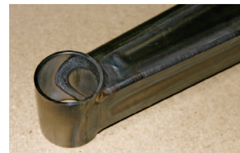
▲ A close look at the shock mounts on the lower link reveals flawless TIG-welding and a simple, effective design.
